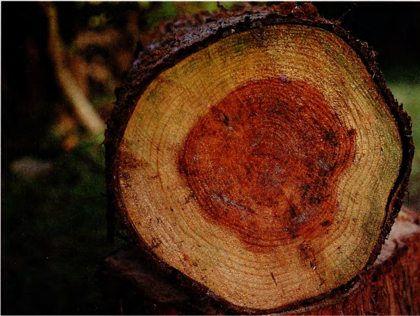
Sapwood and heartwood of 50 year old dawn redwood (Charlottenlund, March 1998). Splint og kerne i 50 år gammel vandgran.
